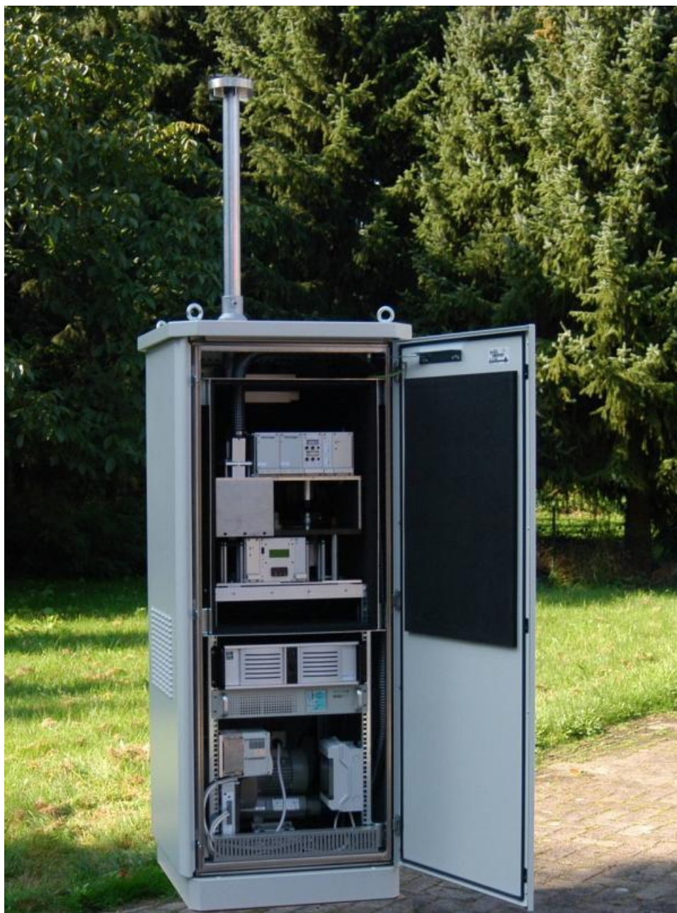
Figure 7: Automatic pollen taxa classification counting station. Source is Fraunhofer-Gesellschaft, Automatic Measuring Stations for Pollen will Improve Forecasts, ScienceDaily , February 12, 2009, http://www.sciencedaily.com/releases/2009/02/090203081615.htm . Last accessed January 28, 2013
